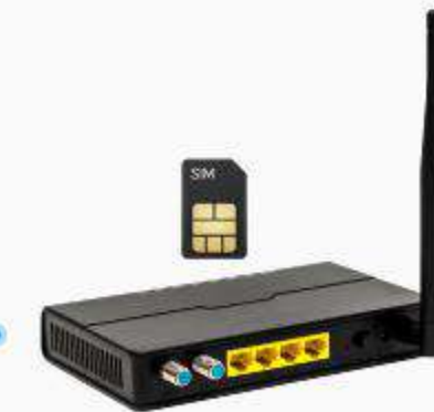
Router with 4G SIM Card
